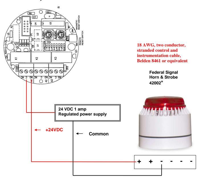
This drawing shows how to connect a remote Horn and strobe to PureAire' LEL monitor with the Alarm Relay #1 set to a Normally Open position.
