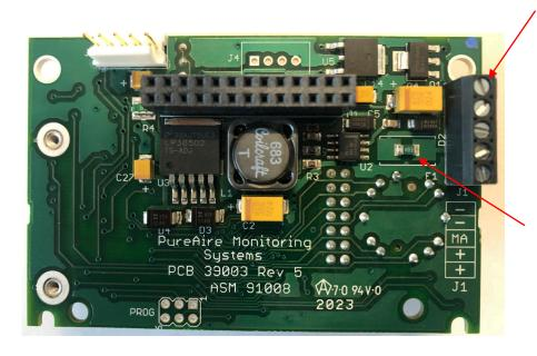
1. Power Analog output Terminal Block
