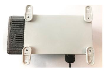
Mounting Feet can be oriented in any direction
