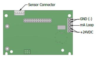
Caution: DO NOT connect to a powered current loop receiver. The Air Check Oxygen monitor supplies the current loop power.
