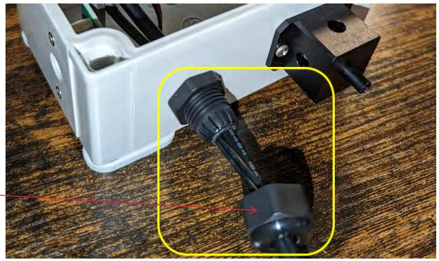
5) Identify the (3) labeled wires on the CloudConnect module, and fee the wires through the cord grip opening, as shown above in Step 4. Do not tighten the cord grip, yet.
