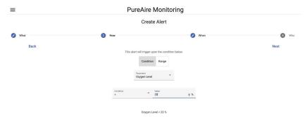
In this example, we are creating an **Oxygen Level Alert**. We set the threshold as "Oxygen Level < 20%".
