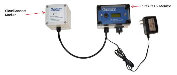
Before logging into the monitoring software, let's get the CloudConnect module all wired up.
