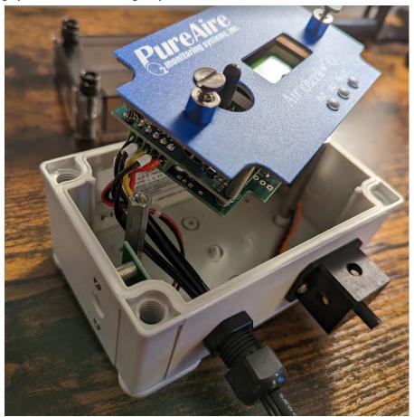
8) Place the electronic board back into position, and hand tighten the (2) flathead screws. Replace the front cover, and hand tighten the (4) Phillips plastic screws. Re-tighten the cord grip. Hardware setup complete!
