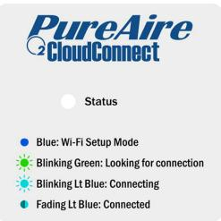
Each CloudConnect module has a status LED that will change color based on the current state.
