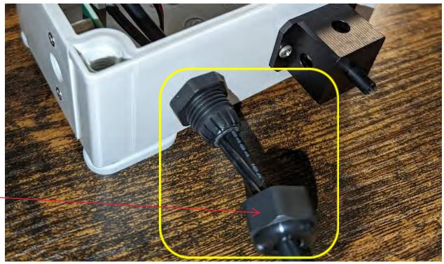
5) Find the (3) labeled wires on the CloudConnect module, and feed the wires through the cord grip opening, as shown above in Step 4. Do not tighten the cord grip, yet.
