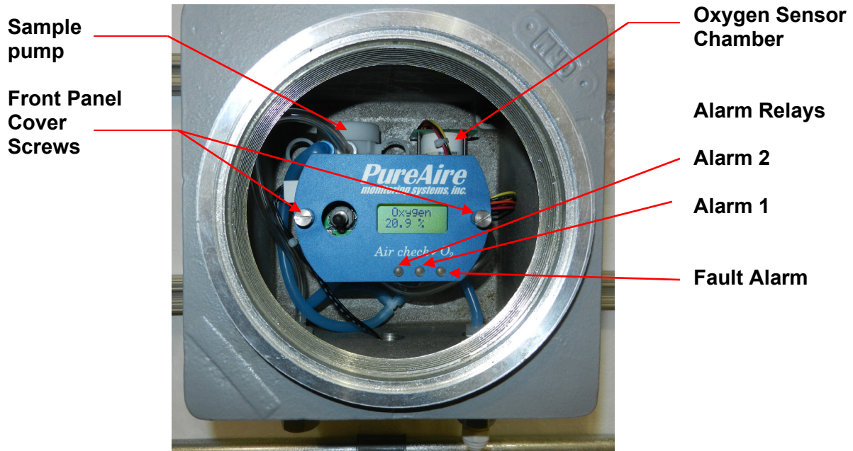
O 2 monitor with front cover removed
