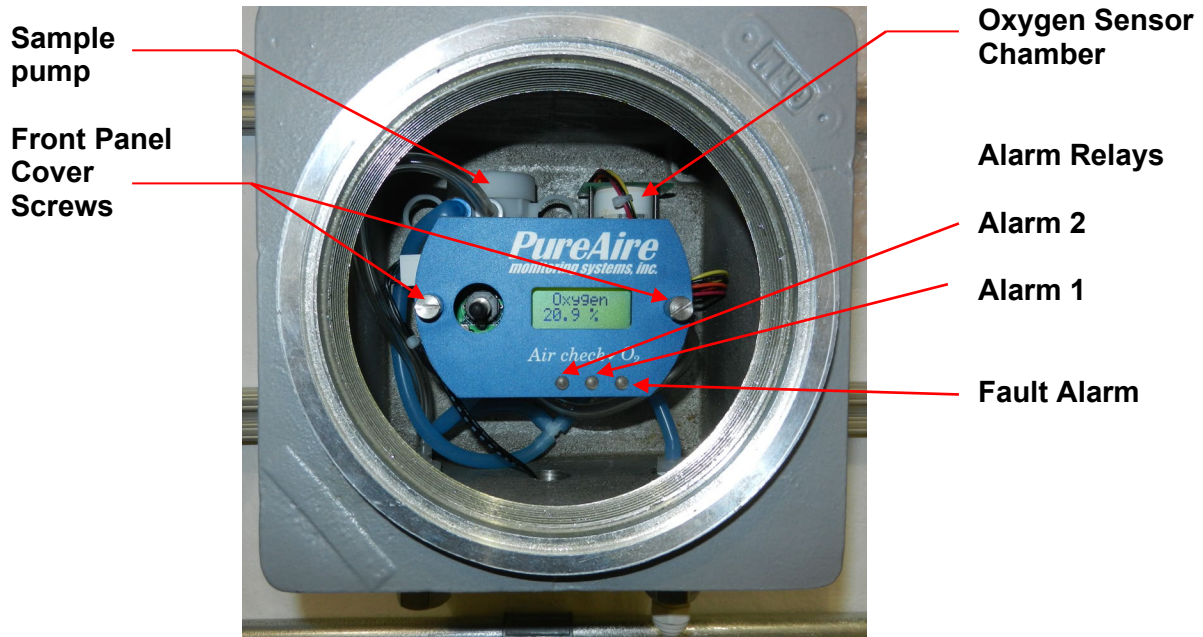
O2 monitor with front cover removed
