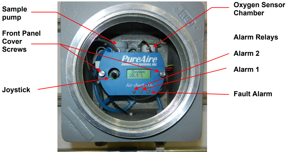
O2 monitor with front cover removed
