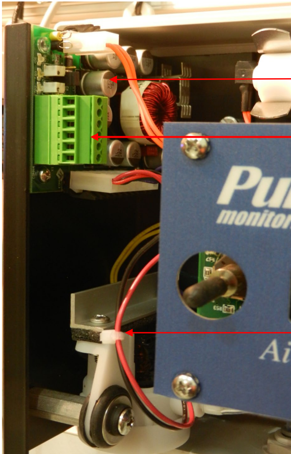
Pump and Pyrolizer Drive Assembly
