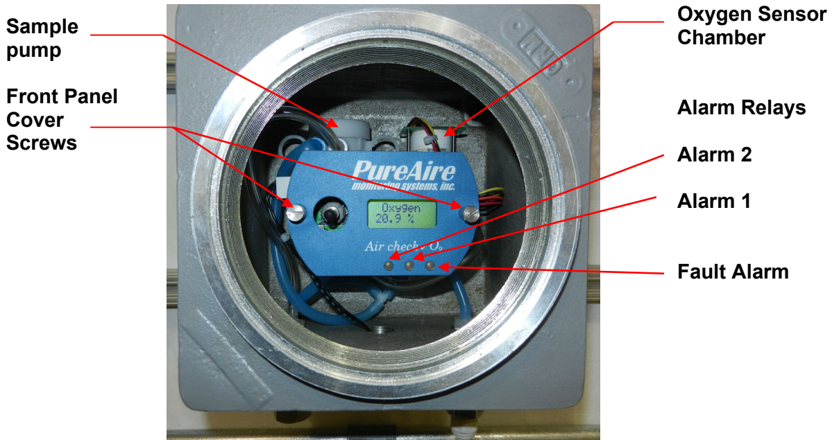
O 2 monitor with front cover removed
